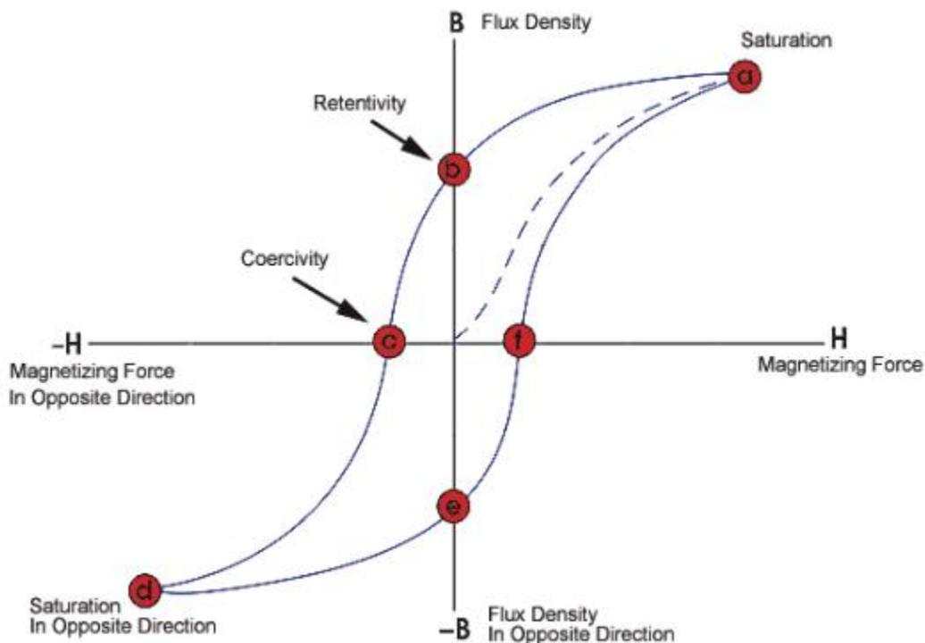
The loop is generated by measuring the magnetic flux of a ferromagnetic material while the magnetizing force is changed. A ferromagnetic material that has never been previously magnetized or has been thoroughly demagnetized will follow the dashed line as **H** is increased. As the line demonstrates, the greater the amount of current applied (**H+**), the stronger the magnetic field in the component (**B+**). At point "**a**"
