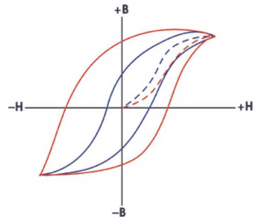
In magnetic particle testing, the level of residual magnetism is important. Residual magnetic fields are affected by the permeability, which can be related to the carbon content and alloying of the material. A component with high carbon content will have low permeability and will retain more magnetic flux than a material with low carbon content.
