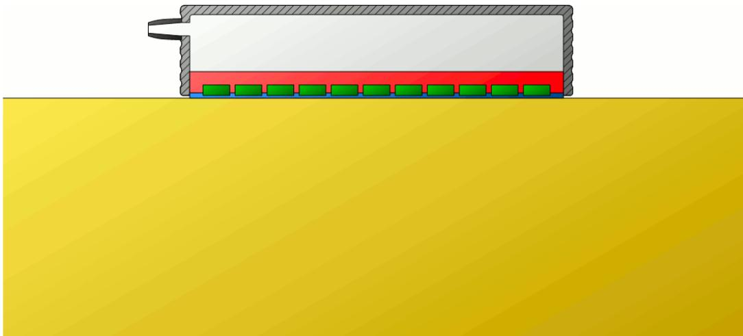
Animation: Phased array probe with inclined intromission of sound
