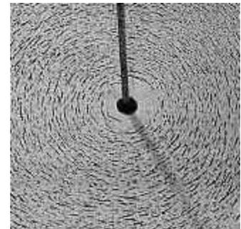
Also, the direction of the magnetic field is dependent on the direction of the electrical current in the wire. The direction of the magnetic field around a conductor can be determined using a simple rule called the "right-hand clasp rule". If a person grasps a conductor in one's right hand with the thumb pointing in the direction of the current, the fingers will circle the conductor in the direction of the magnetic field.
