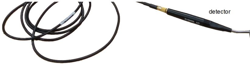
Figure: Measuring tool for eddy current testing
