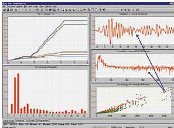
Also common to most AE systems is the ability to perform routine tasks that are valuable for AE inspection. These tasks include quantitative signal measurements with corresponding time and/or load readings, discrimination between real and false signals (noise), and the collection of statistical information about the parameters of each signal.
