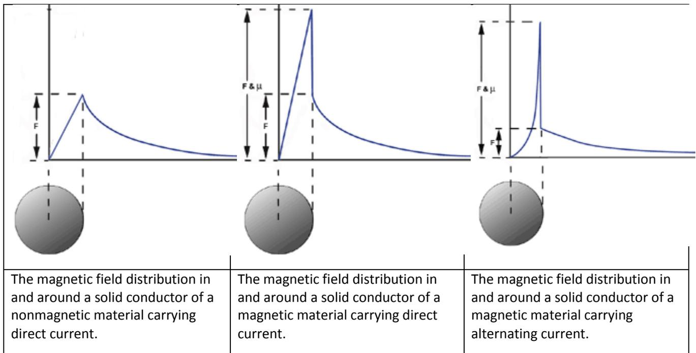
In a hollow circular conductor there is no magnetic field in the void area. The magnetic field is zero at the inner surface and rises until it reaches a maximum at the outer surface.
