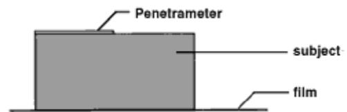
Image quality indicators take many shapes and forms due to the various codes or standards that invoke their use. The two most commonly used IQI types are: the hole-type and the wire IQIs. IQIs come in a variety of material types so that one with radiation absorption characteristics similar to the material being radiographed can be used.
