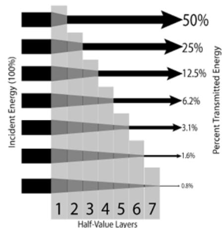
Sometimes instead of specifying the **HVL**, the Tenth Value Layer (**TVL**) is specified. The **TVL** is the thickness that attenuates 90% of the intensity (only 10% passes through).
