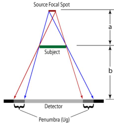
The angle between the radiation and some features will also have an effect on definition. If the radiation is parallel to an edge or linear discontinuity, a sharp distinct boundary will be seen in the image. However, if the radiation is not parallel with the discontinuity, the feature will appear distorted, out of position and less defined in the image.
