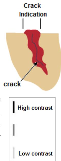
Liquid penetrant testing is one of the most widely used NDT methods. Its popularity can be attributed to two main factors: its relative ease of use and its flexibility. It can be used to inspect almost any material provided that its surface is not extremely rough or porous. Materials that are commonly inspected using this method include; metals, glass, many ceramic materials, rubber and plastics.
