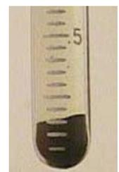
2.4 ml for visible particles. If the particle concentration is out of the acceptable range, particles or the carrier must be added to bring the solution back in compliance with the requirement.
