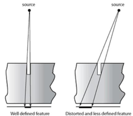
Abrupt changes in thickness and/or density will appear more defined in a radiograph than will areas of gradual change. For example, consider a circle. Its largest dimension will be a cord that passes through its centerline. As the cord is moved away from the centerline, the thickness gradually decreases. It is sometimes difficult to locate the edge of a void due to this gradual change in thickness.
