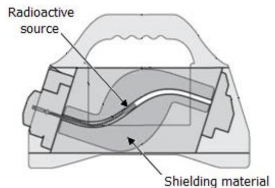
To make a radiographic exposure, a crank-out mechanism and a guide tube are attached to opposite ends of the exposure device. The guide tube often has a collimator (*usually made of tungsten*) at the end to shield the radiation except in the direction necessary to make the exposure.
