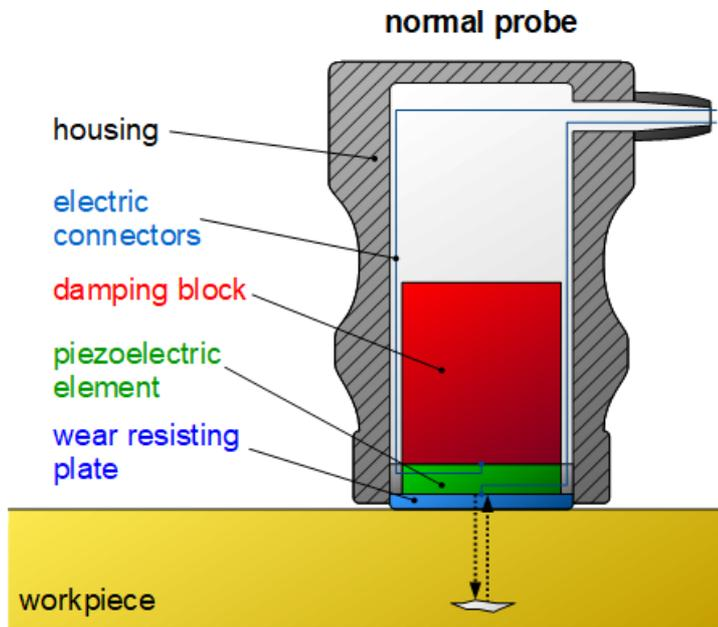
Figure: Components of a normal probe
