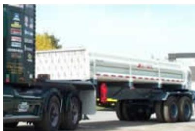
each end. A multichannel acoustic system is used to detection and mapped source locations. Suspect locations are further evaluated using ultrasonic inspection, and when defects are confirmed the tube is removed from use. AET can detect subcritical flaws whereas hydrostatic testing cannot detect cracks until they cause rupture of the tube. Because of the high stresses in the circumferential direction of the tubes, tests are geared toward finding longitudinal fatigue cracks.
