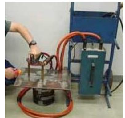
However, caution is required when using prods because electrical arcing can occur and cause damage to the component if proper contact is not maintained between the prods and the component surface. For this reason, the use of prods is not allowed when inspecting aerospace and other critical components. To help prevent arcing, the
