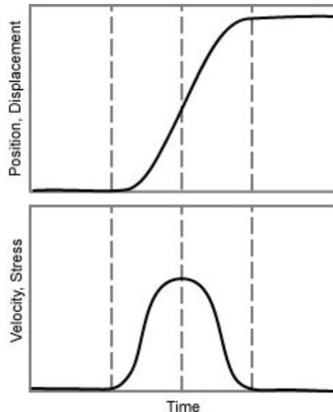
Primitive AE wave released at a source. The primitive wave is essentially a stress pulse corresponding to a permanent displacement of the material. The ordinate quantities refer to a point in the material.
