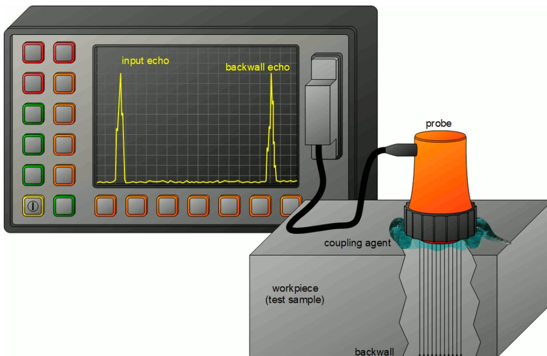
Figure: Principle of ultrasonic testing
