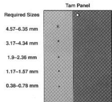
Care of system performance check specimens is critical. Specimens should be handled carefully to avoid damage. They should be cleaned thoroughly between uses and storage in a solvent is generally recommended. Before processing a specimen, it should be inspected under UV light to make sure that it is clean and not already producing an indication.
