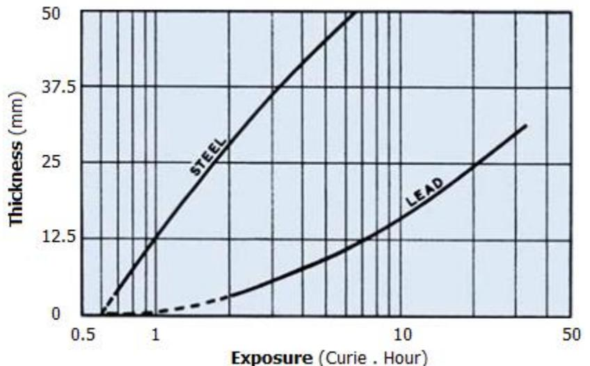
It should be noted that such charts are valid for the specified parameters, but of course using the data in the charts one can calculate the exposure for different set of parameters such as different source-to-film distance, different type of film, or different density.
