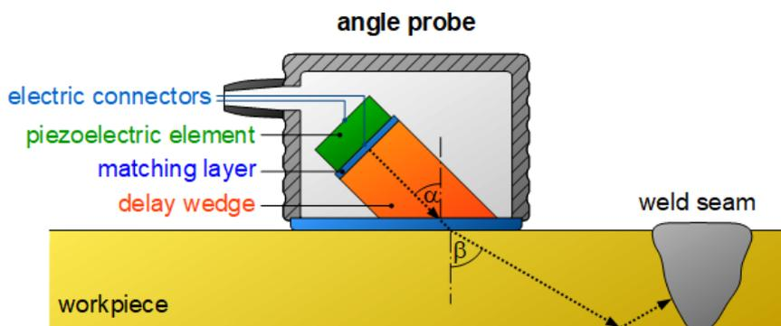
Figure: Components of an angle probe
