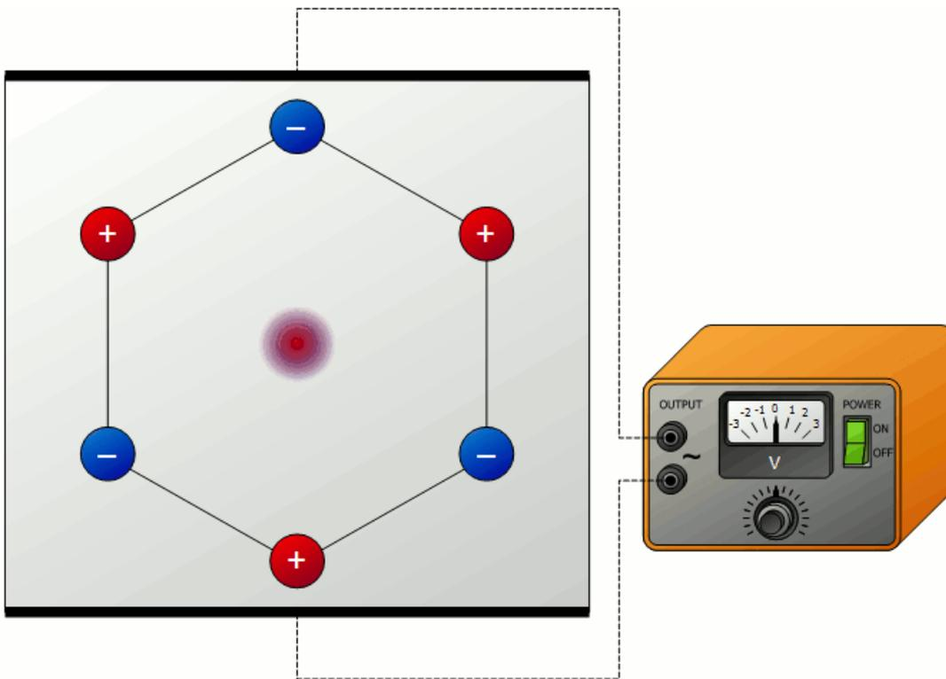
Animation: Piezoelectric crystal on an alternating voltage
