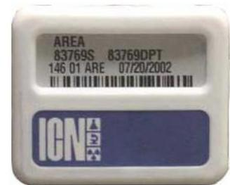
The film is contained inside a film holder or badge. The badge incorporates a series of filters to determine the quality of the radiation. Radiation of a given energy is attenuated to a different extent by various types of absorbers. Therefore, the same quantity of radiation incident on the badge will produce a different degree of darkening under each filter. By comparing these results, the energy of the radiation
