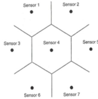
When additional sensors are applied, arrival times and amplitudes help pinpoint the source zone. The ordered pair in lower right figure represents the two sensors detecting the signal in the zone and the order of signal arrival at each sensor. When relating signal strength to peak amplitude, the largest peak amplitude is assumed to come from the nearest sensor, second largest from the next closest sensor and so forth.
