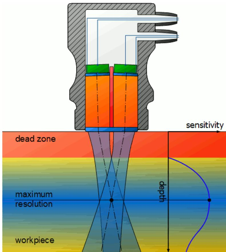
Figure: Dead zone and sensitivity of a TR probe
