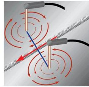
Magnetization Using Indirect Induction (Indirect Magnetization)
