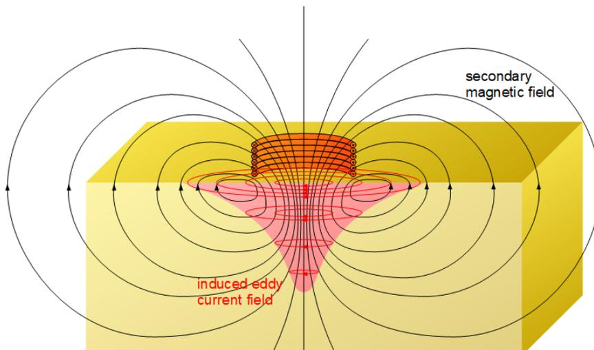
Figure: Secondary magnetic field induced by eddy currents
