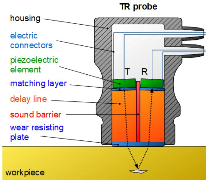
Figure: Components of a TR probe
