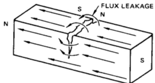
If iron particles are sprinkled on a cracked magnet, the particles will be attracted to and cluster not only at the poles at the ends of the magnet, but also at the poles at the edges of the crack. This cluster of particles is much easier to see than the actual crack and this is the basis for magnetic particle inspection.
