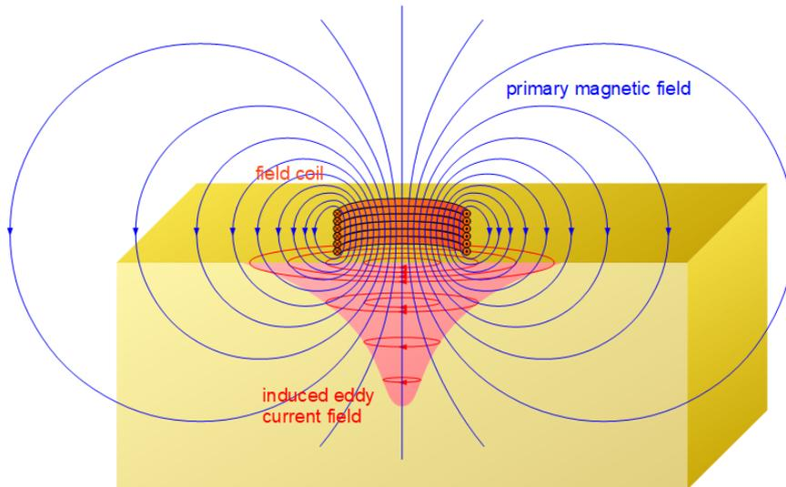
Figure: Induction of eddy currents by primary magnetic field
