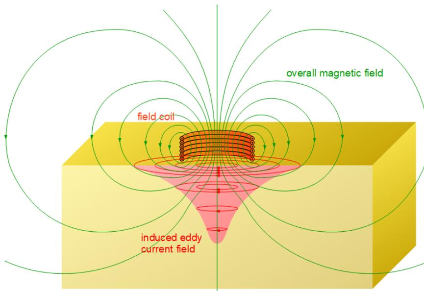
Figure: Overall magnetic field as superposition of primary and secondary field
