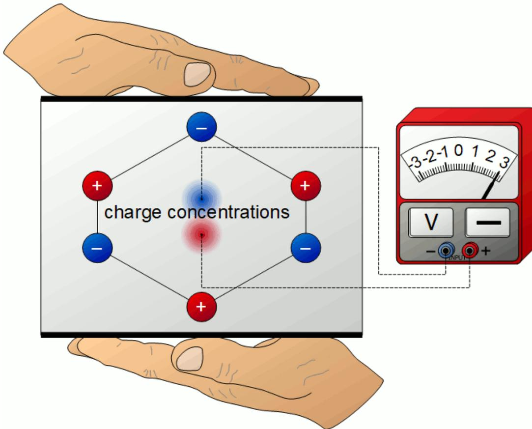
Figure: Piezoelectric effect
