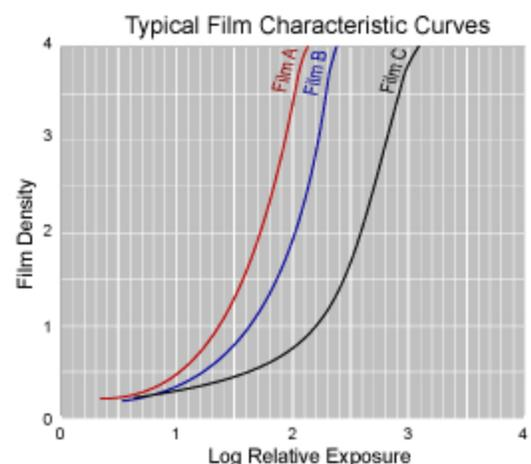
example, if one film is exposed at  $100\text{ kV}$  for  $6\text{ mA}\cdot\text{min}$  and a second film is exposed at the same energy for  $3\text{ mA}\cdot\text{min}$ , then the relative exposure would be 2.
