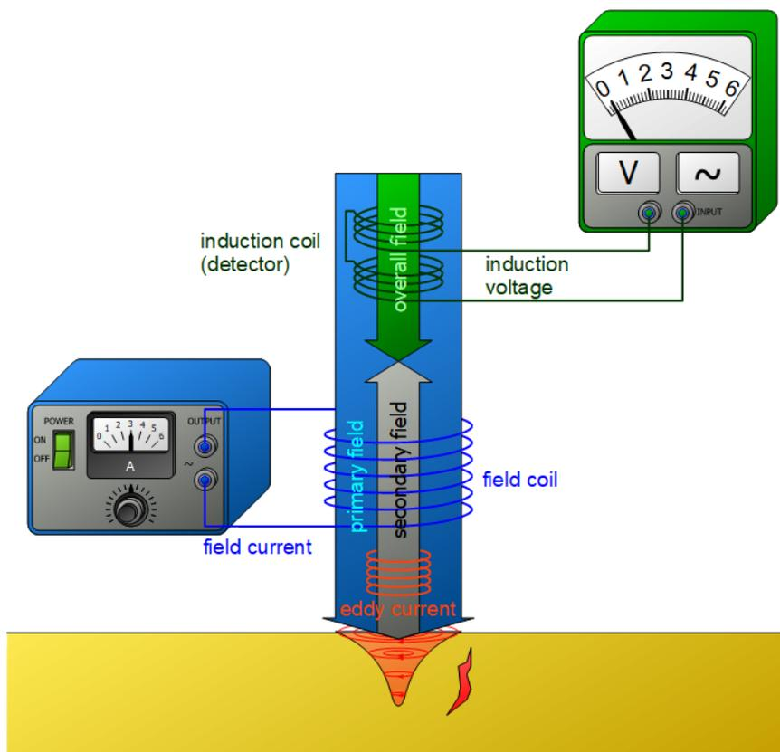
Figure: Principle of eddy current testing
