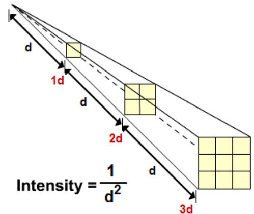
As one of the fields which obey the general inverse square law, the intensity of the radiation received from a point radiation source can be characterized by the diagram above. The relation between intensity and distance according to the inverse square law can be expressed as:
