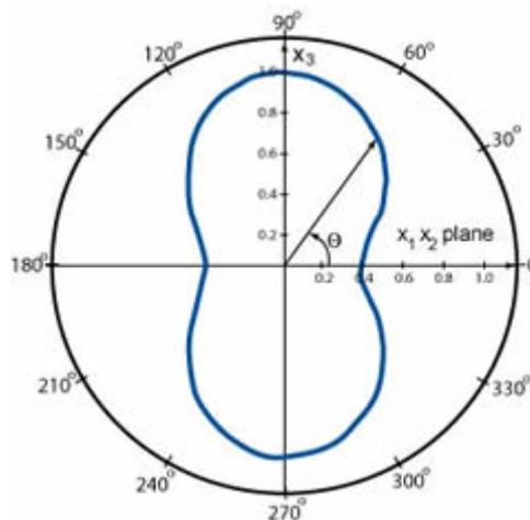
Angular dependence of acoustic emission radiated from a growing microcrack. Most of the energy is directed in the 90 and 270° directions, perpendicular to the crack surfaces.
