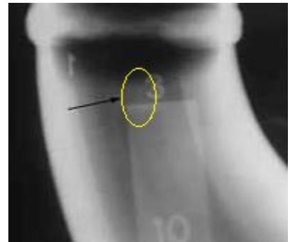
The control of backscatter radiation is achieved by backing the film in the cassette with a sheet of lead that is at least *0.25 mm* thick such that the sheet will be behind the film when it is exposed. It is a common practice in industry to place thin sheets of lead (called "lead screens") in front and behind the film (*0.125 mm thick in front and 0.25 mm thick behind*).
