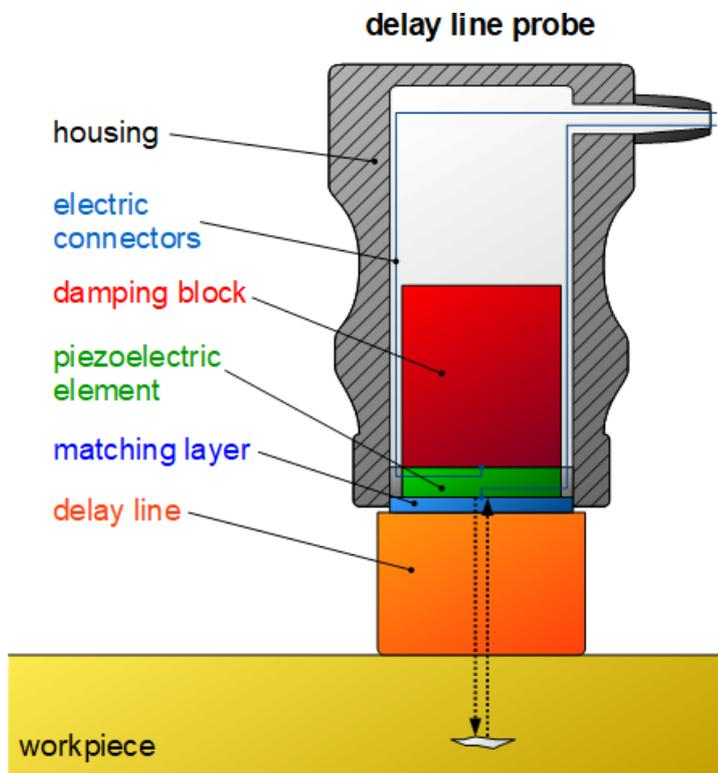
Figure: Components of a delay line probe
