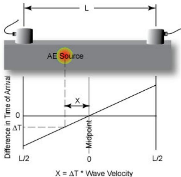
Because the above scenario implicitly assumes that the source is on a line passing through the two sensors, it is only valid for a linear problem. When using AE to identify a source location in a planar material, three or more sensors are used, and the optimal position of the source is between the sensors. Two categories of source location analysis are used for this situation: zonal location and point location.
