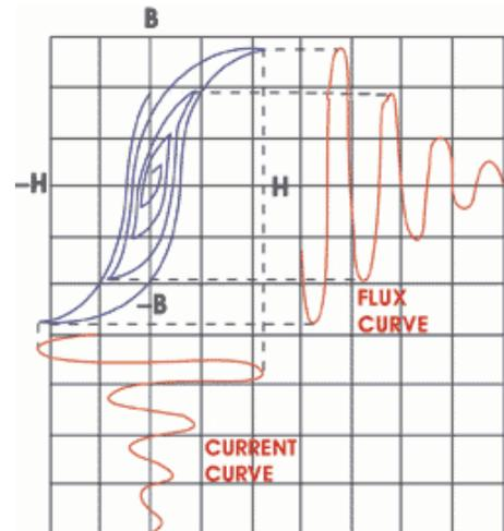
A field meter is often used to verify that the residual flux has been removed from a component. Industry standards usually require that the magnetic flux be reduced to less than 3 Gauss ( $3 \times 10^{-4}$  Tesla) after completing a magnetic particle inspection.
