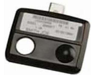
A *TLD* has a phosphor, such as lithium fluoride (LiF) or calcium fluoride (CaF), in a solid crystal structure. When a *TLD* is exposed to ionizing radiation at ambient temperatures, the radiation interacts with the phosphor crystal causing some of the atoms in the material to produce free electrons and become ionized. The free electrons are trapped and locked into place in the imperfections in the crystal lattice structure.
