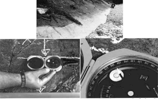
•Compass must be horizontal (bull's eye bubble centered), with compass edge flush to the tilted plane
