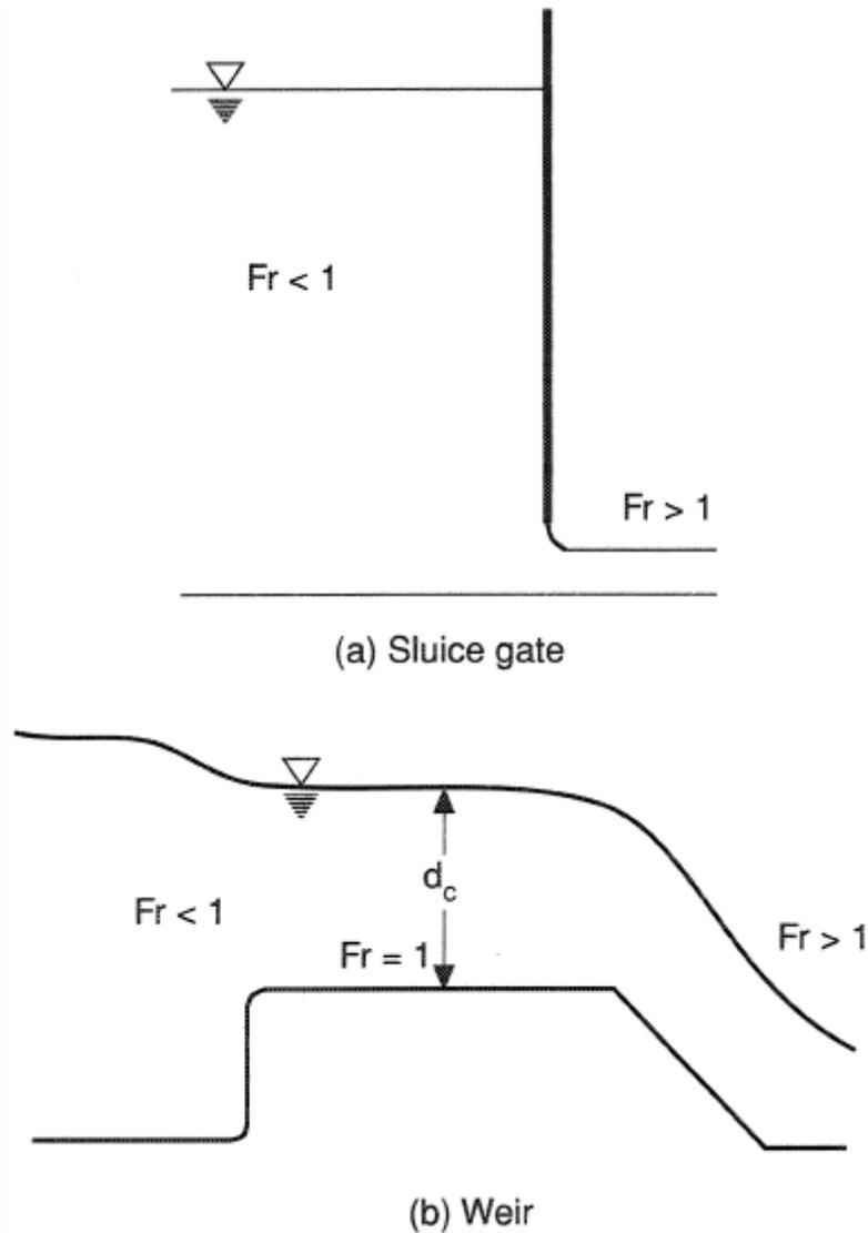
Figure 3. Open channel control structures.
