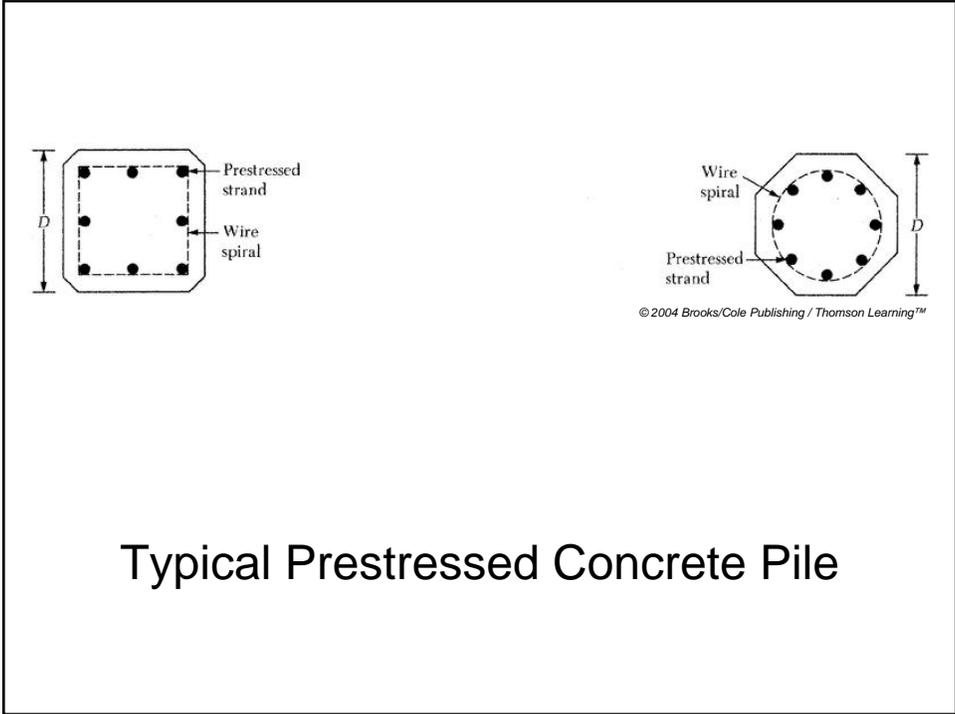
Typical Prestressed Concrete Pile
