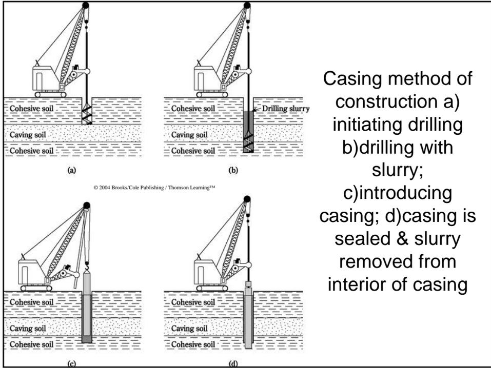
Casing method of construction
