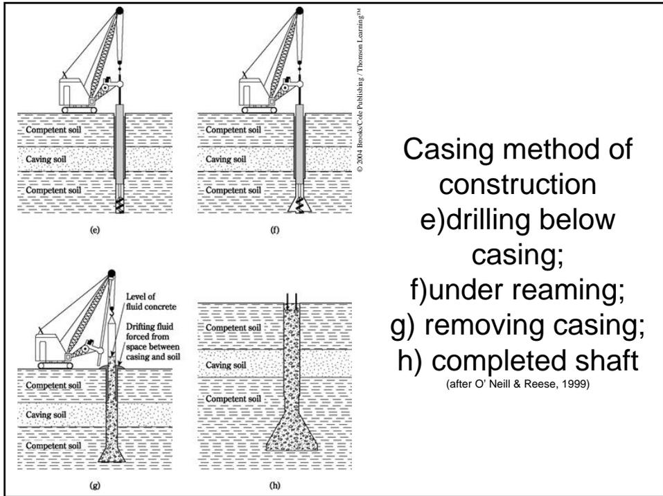
Casing method of construction
